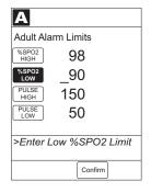
6. To confirm alarm settings and return to **SPO2 Main** display, press **Confirm** soft key.
